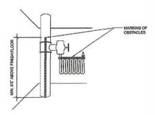
For compliant placement of obstacle markings, consult your applicable local or national codes (2009, 2012 IBC section 1024 +2015 IBC section 1025).
