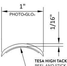
Photo-Glo® is made of the same industrial grade solid polymer used in golf balls with imbedded glow-in-the-dark pigment. This creates a durable material that is approximately 50% brighter than the code requires. Photo-Glo comes with an industry leading 25-year warranty.
