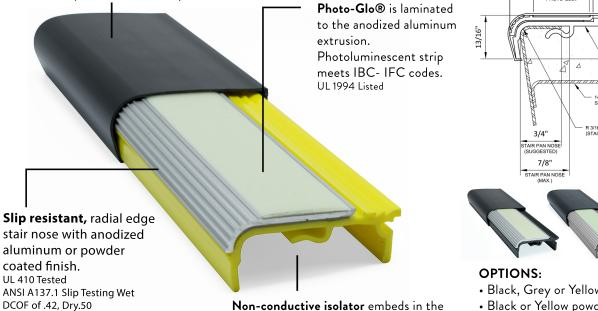
Four piece design: 2" non-conductive pvc isolator, replaceable anodized nosing, replaceable 1" Photo-Glo® strip, patented construction cover. Assembly clips on prior to concrete pour. Up to 12', to the nearest 1/16''.
